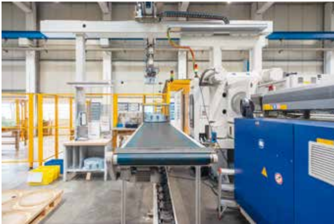
The injection moulding machines dispense the products on the operator side - the finished parts to the clamping side, the QA parts to the injection side. The larger machines have a feeder for the insert bushings (under the conveyor belt).
