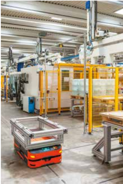
The vehicles orient themselves on fixed magnetic strips placed at right angles on the floor. They can turn on the spot. Each vehicle has its own parking position for recharging its batteries.
