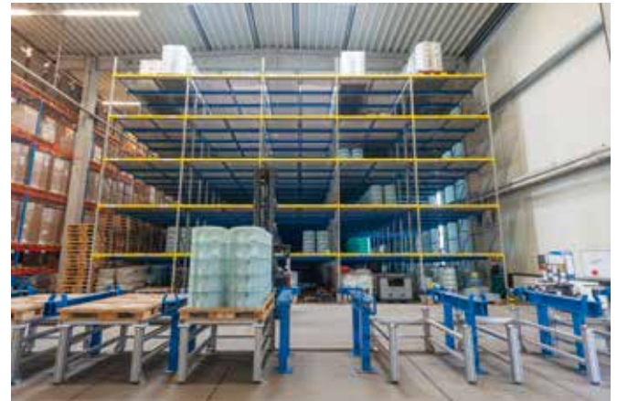
At the station (in the foreground) in front of the buffer warehouse, the driverless transport system sets down filled pallets and picks up empty pallets. On the opposite side, a forklift takes over and lifts them into the buffer warehouse.
